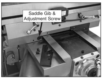
Figure 63. Saddle gib and adjustment screw.
